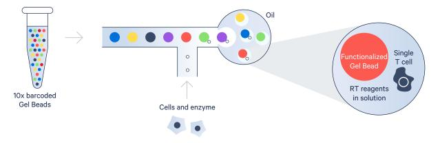
**Next GEM technology and single cell partitioning.** Using advanced microfluidics, Chromium Single Cell instruments encapsulate Gel Beads in GEMs, or a "Gel Bead-in-emulsion," along with uniquely barcoded single cells or nuclei and reagents to create a micro-reaction.
